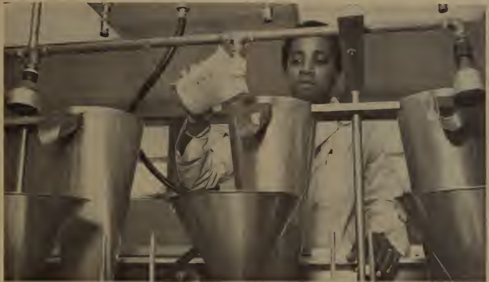
Testing in Cooper Lab -- This is the way you extract nematodes from soil samples. That is what Horacena Taylor, agricultural science assistant II, is doing here in the nematode assay section of the Agricultural Service Laboratory. The laboratory was recently named to honor the memory of H.P. Cooper, an agronomist and educator whose career with the College of Agricultural Sciences here spanned 60 years. Robert Lippert is the new director of the lab.
